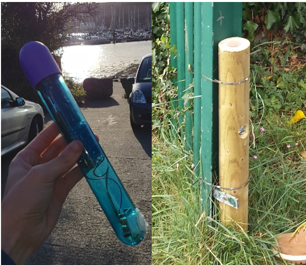
Figure 2 & 3. Inner and Outer layers of enclosure
